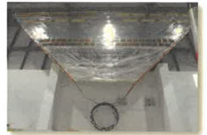
Sail from IKAROS, a solar powered space kite [3]
