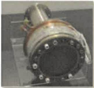
Ion engine tested for continuous operation [3]
